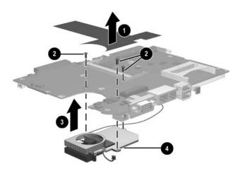
Removing the Fan and Heat Sink
